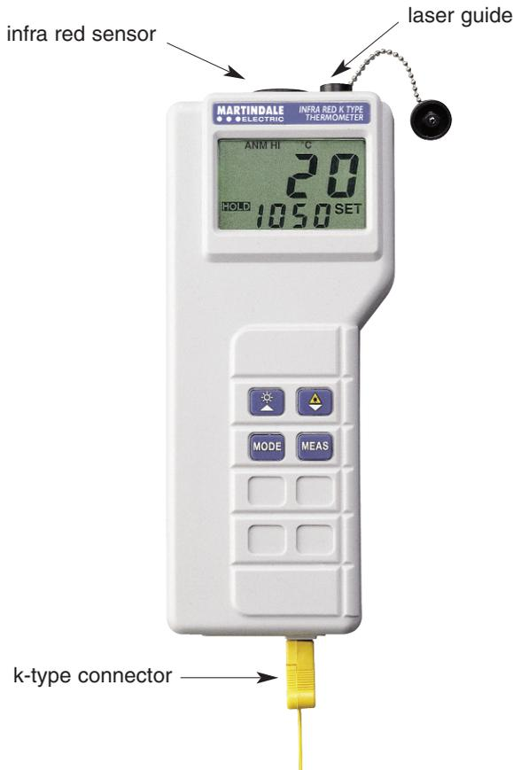
This thermometer has a laser marker to ensure accurate spot measurement. The display can show temperatures in Fahrenheit or Celsius. A limit function sets upper and lower thresholds and a tone alerts if they are exceeded. Optional auto power off conserves battery life. The emissivity can be adjusted for different surfaces. K Type thermocouples can be used and comes with it.
